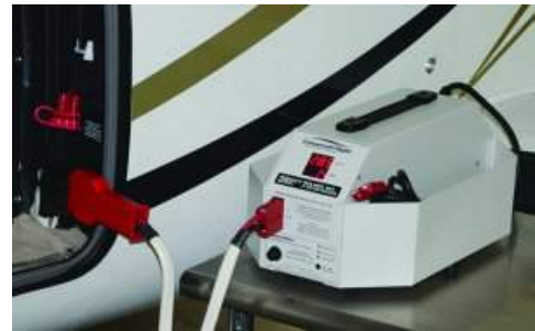
In between servicing, use ground power for extended engine-off operation. That's an Enhanced Flight portable GPU.
