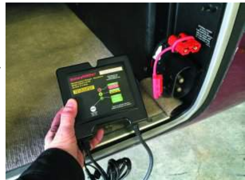
Since aircraft batteries aren't easy to access, a plug for connecting a battery tender will make your life much easier. The Enhanced Flight connector kit for VDC chargers is approved for permanent installations.
