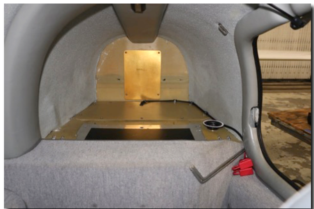
Aft baggage interior with trim removed.
