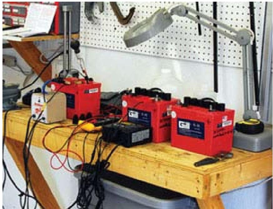
The lab. Not seen is the computer for logging the data or the temperature compensated hydrometer for measuring the specific gravity. At far left is what was thought to be a safe 1-amp charger. **The black box is the Battery Minder from VDC**; the yellow box is the digital voltmeter.
