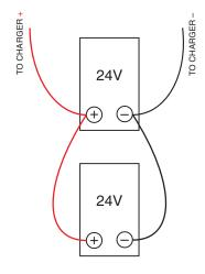
24 VOLT (Parallel Connected) = 24V
