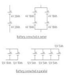
Connect each battery to one another using 18 gauge (lamp cord type) insulated wire. Strip at the points where you wish it to be in electrical contact with the posts of each battery, then use ring or clip connectors. VDC Electronics, Inc. does not provide any type of wire harness to accomplish this, due to the many variations in size and terminal configuration.
