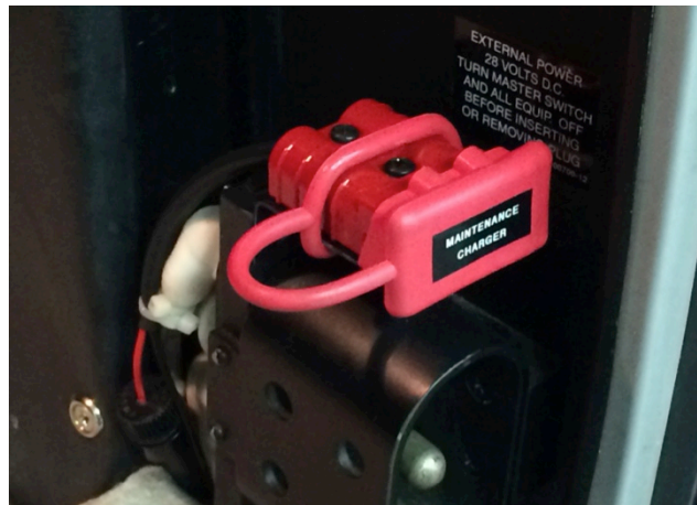
Maintenance charger plug & cover installed.
